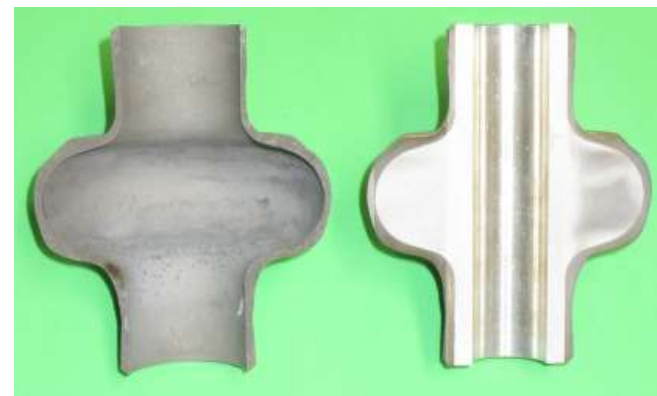
Cavity model made by cold spray
