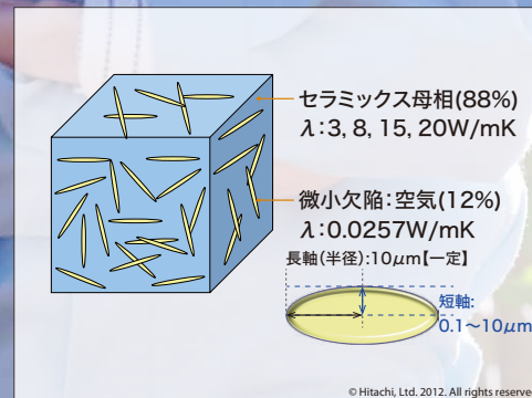
溶射膜の解析形状モデル Analysis geometric model of sprayed coating.
