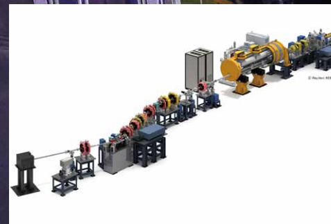
超伝導加速器とその出力電子ビームを細く絞るビームラインとX線生成装置の模式図 Illustration of the superconducting accelerator, the beam line for squeezing its transverse size, and the X-ray generation section
