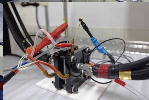
MEAを利用した単電池 Single cell unit with MEA
